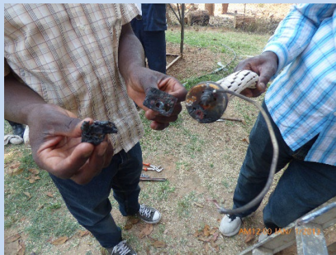
Water geyser burned out thermostat and heating element
